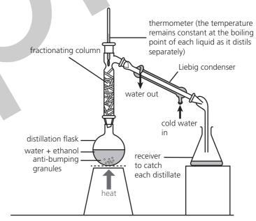
Simple **fractional distillation** can be carried out in the laboratory using the equipment shown.
